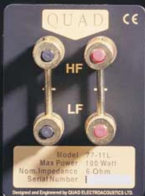
The gold-plated terminals offer the facility of bi-wiring. Even if your amplifier has only one set of loudspeaker terminals, significant sonic advantages can be gained by using a good quality bi-wire cable, linking them at the amplifier end, but separating them at the loudspeaker end. This reduces the intermodulation effects and improves the 'openness' and clarity of the speaker still further.
