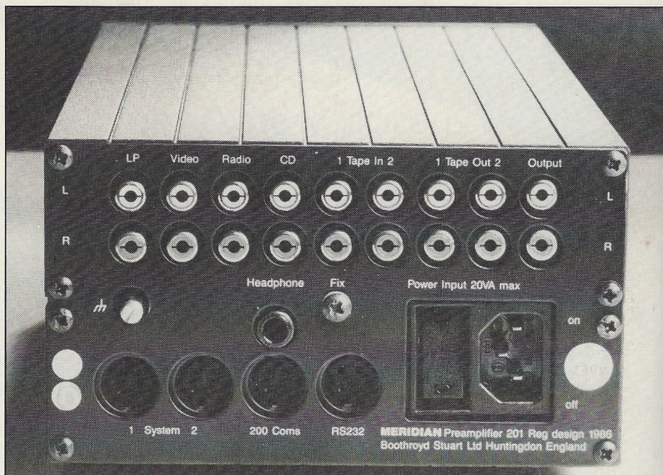
Flexibility is the keynote, with six inputs and the ability to feed two systems
