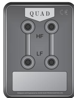
The crossover separates the treble and bass networks into two distinct sections, each connected by a dedicated pair of terminal posts. This enables the treble and bass components to be separately driven for optimum performance. The upper pair of terminals is connected to the treble network and the lower pair to the bass network. As supplied, the treble terminal pair is connected to the bass terminal pair by removable metal straps. These should be left in place for standard installations.
