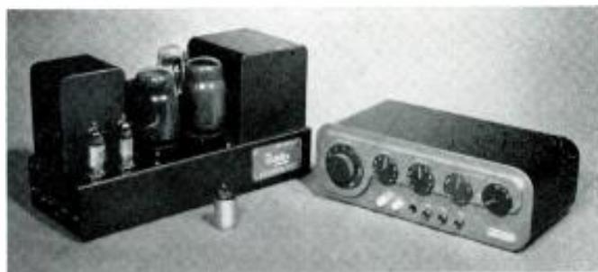
*Quad II amplifier, quality control unit, pickup matching plug.*
