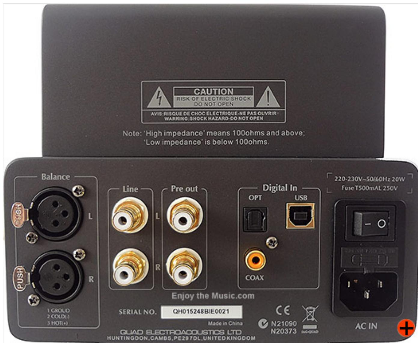
On the back you will find one balanced input (pin 3 running "hot"), one line input and the single ended pre out along with the aforementioned digital inputs. Also on the back the power switch and IEC power inlet, all clean and tidy arranged.
