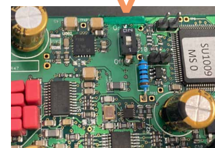
Switch set to "On" – Signal Sense enabled
