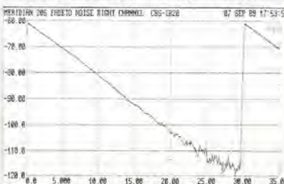
Fig 4. Meridian 206. linearity plot below -60dB
