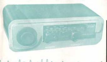
A superheterodyne circuit is used. There are three controls, Tuning, Waveband and Selectivity. The edge-lit dial is calibrated in metres and carries the names of B.B.C. stations. An electronic tuning indicator of the latest type is fitted, to permit accuracy of tuning, an essential in high quality equipment.
